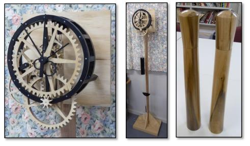
A beautifully constructed long case skeleton clock made by Lionel Wood. Pendulum operated, this clock is mostly scroll-sawn from marine plywood for durability and took several months to complete. A set of veerrry large pepper and salt grinders made by John Hatton from Tulip Wood. These would not be out of place over the shoulder of a waiter in a very fancy restaurant.
